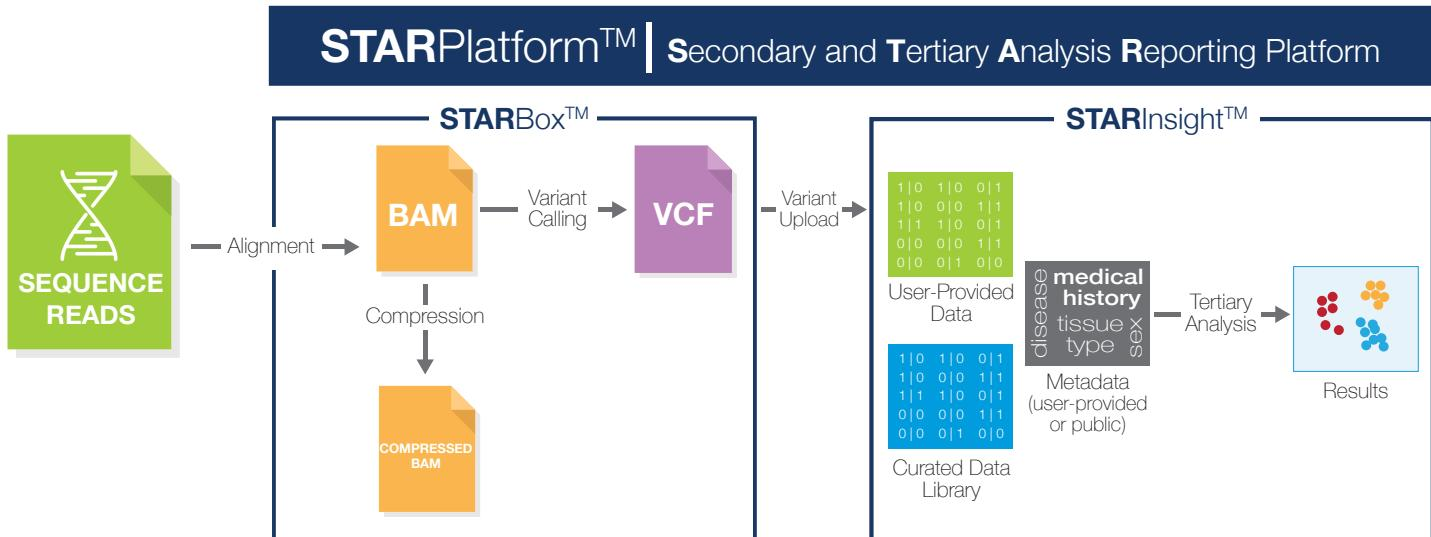
**STAR**Box performs two distinct workflows on sequence reads: secondary analysis and compression. During secondary analysis, the system aligns the sequence reads, performs variant calling, and creates a VCF file. The aligned sequence reads are quickly compressed using Annai's industry-leading lossless technology. **STAR**Box can send processed files to a repository of your choice.
